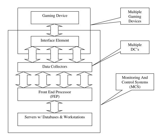
In the illustration above, this standard applies to all components referenced other than the Gaming Device. The requirements for the Gaming Device are defined in the applicable Device Standard. This document will only concern communications from the Gaming Device to the MCS, and not in the reverse order, with the exception of the Ticket/Voucher Validation System Requirements that are incorporated within Chapter 4.
